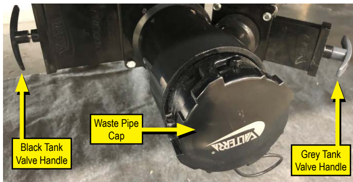
Example of Tank Drain Located Underneath RV
