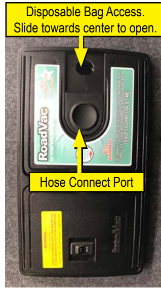
Cargo Area Vacuum Access
