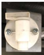
Exterior Fresh Water Drain Example
