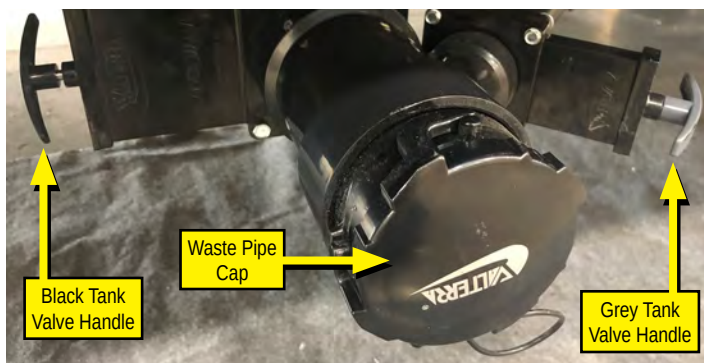
Example of Tank Drain Located Underneath RV
