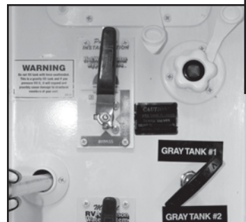
Water Heater Bypass (One Valve System)
