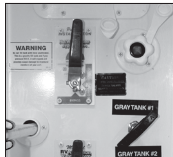
Water Heater Bypass (One Valve System)
