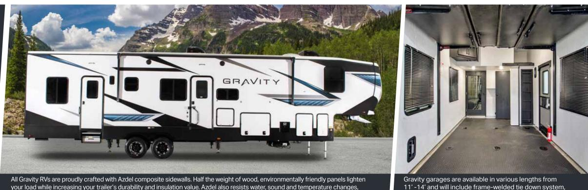
your load while increasing your trailer's durability and insulation value. Azdel also resists water, sound and temperature changes, keeping your living spaces comfortable and quiet.
