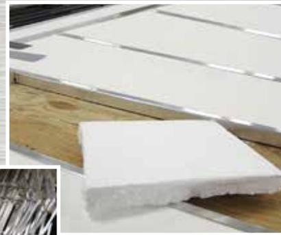
A 1/8" thin coffee cup can protect your hand from scalding hot coffee - consider the protection Heartland's sidewalls offer featuring 1.5" block foam insulation
