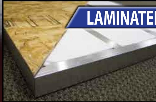
XLT's LAMINATED Floor System is one of the **STRONGEST FLOORS** in the industry! Featuring sturdy 2.5" Aluminum Framing; thick Block Foam Insulation; One-Piece Seamless Decking and a Thermo-Board Luan on the bottom. All of this is Laminated together for Maximum Strength and Insulation R Value - virtually eliminating flex in the floor!
